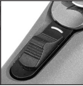
Figure 6. Safety selector in “ SAFE ” position (middle position with one white bar visible). When the safety selector is in this position the bolt handle can be raised.
